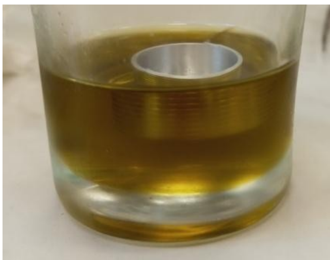
Figure 7. Photograph of the process of determining the density of oil using swimming standard of density
